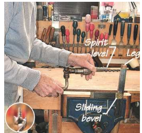
▲ Pic. 7 Here's the set-up for drilling the top rail mortise holes
